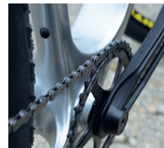
Top: Cheaper SRAM Apex gearing still works fine. Hydraulic brake levers are an Apex option but aren't fitted Bottom: The Cutthroat comes with a single 36t chainring but can be fitted with a double
