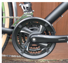
Above: A triple chainset makes it easy to ride at a consistent cadence. Smaller rings would be nice on tour
